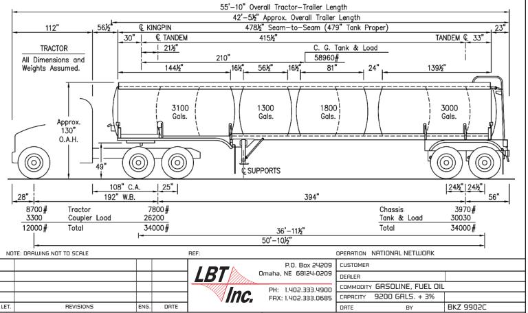
CHASSIS FRAME - Aluminum huck bolted to tank frame rails UNDERCONSTRUCTION - Hendrickson AANT Intraax with "HP" spindles BRAKE SYSTEM – Haldex 4S/2M ABS with "TRS" system **HUBS & DRUMS** – Walther EMC Dura-Light with cast drums WHEELS – (8) 22.5 x 8.25 Aluminum, (4) machine finish, (4) polished TIRES - (8) 11R22.5 (G) trailer type FENDERS – Aluminum front and rear with rubber bushed mountings
